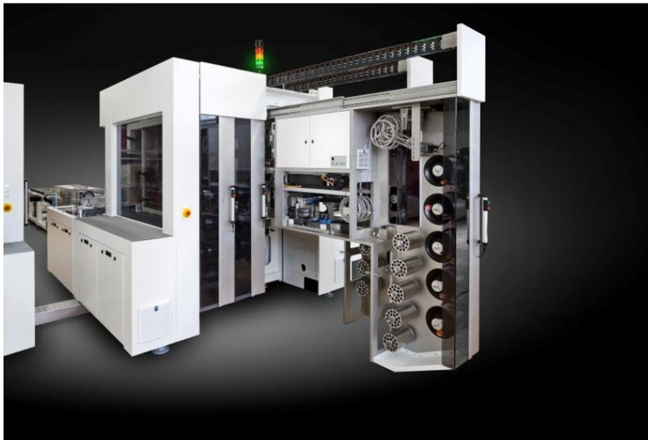
Ribbons can be exchanged at any time without interrupting ongoing production.
